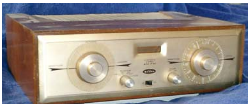
(left) Scott 330C AM/FM simulcast receiver (which required connection to a stereo amplifier and speakers). Note the separate AM and FM tuning dials. (WSMB collection)
